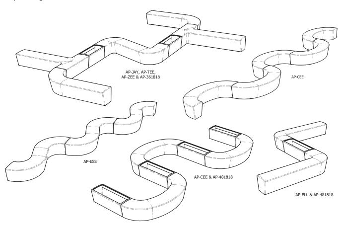
Note: All letter benches are 96" long. Benches are available with hidden internal or exterior anchor brackets - see product drawings for details. Products are treated with medium duty sealant. Planters will be delivered with drain holes unless otherwise specified. Optional skate deterrents to be installed in the field.
